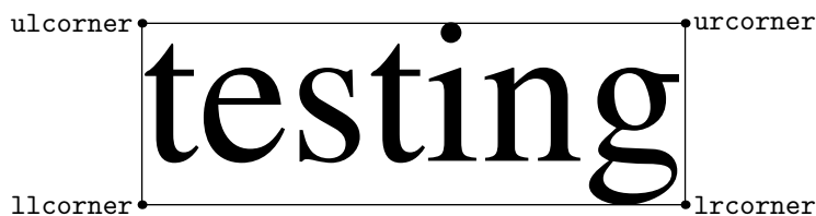
Figure 20: A bounding box and its corner points.
